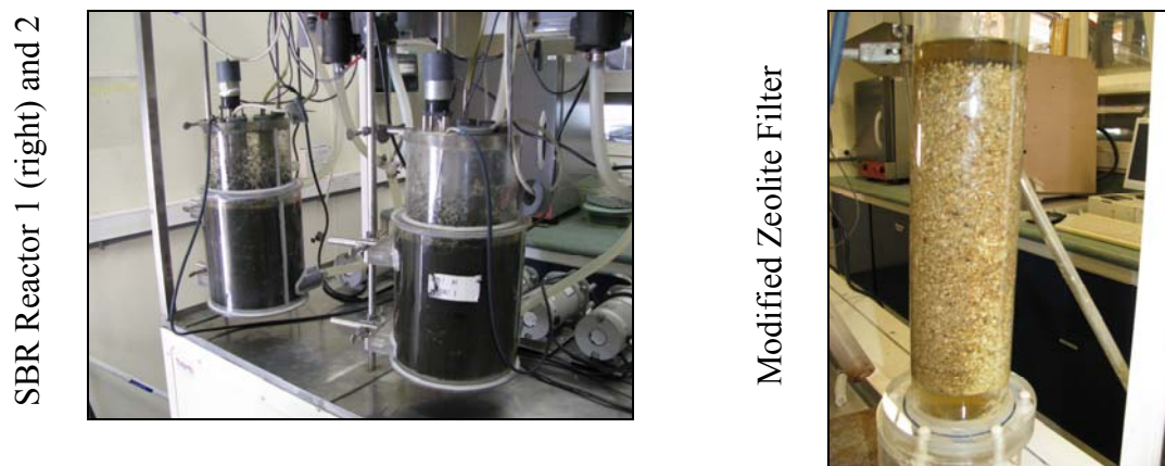
Figure 4. SBR reactors and modified zeolite filter.
